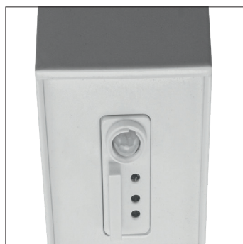
XC daylight&occ sensor
